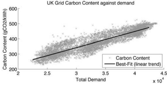
**Figure 3: UK Carbon emission from Electricity Generation.**
